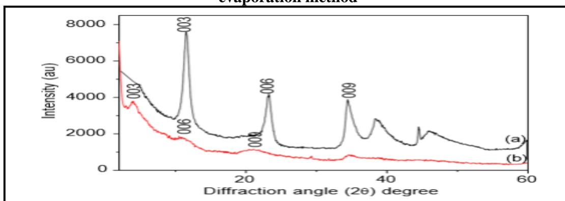
Figure No.4: Powder X-ray diffraction patterns of (a) pristine LDH (sample A) and (b) LDH- MTX (sample B) nanohybrids
