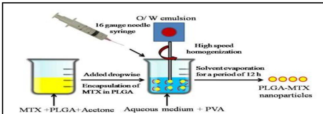
Figure No.3: Development of PLGA-MTX nanoparticles by O/W single emulsification- solvent evaporation method
