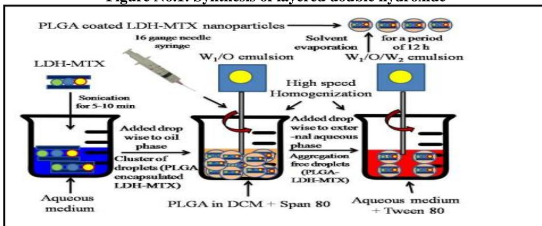
Figure No.2: Optimized technique for synthesis of PLGA-LDH-MTX nanohybrids by W1/O/W2 double emulsion- solvent evaporation method
