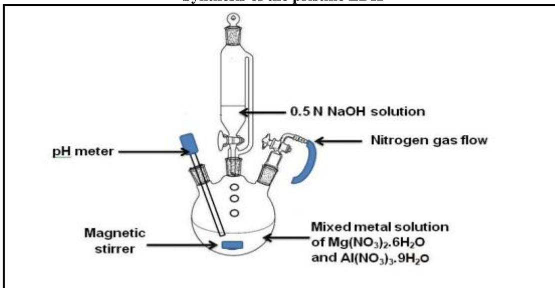
Figure No.1: Synthesis of layered double hydroxide
